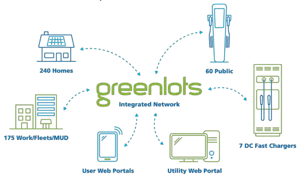
Figure 6: Integrated EVSE network design for the EVSE pilot (2016–2019)
